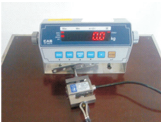
Fig. 14. The device for registering the value of loading with a tensometric sensor
