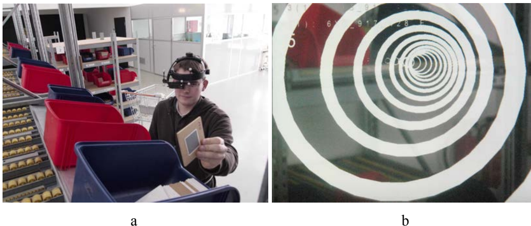
Figure 1. User working with a MAR system: Liteye Head Mounted Display, infrared tracking, AR funnel navigation.
